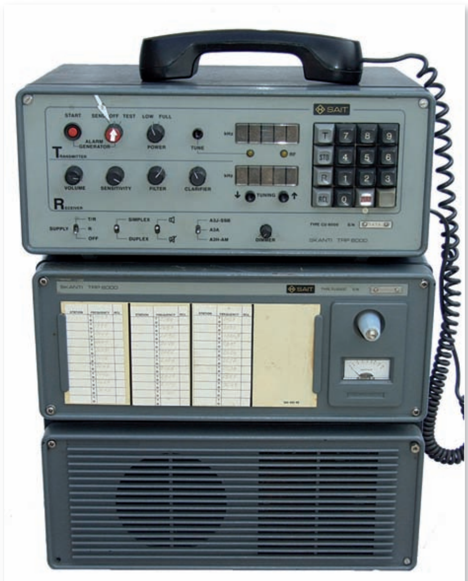
Fig. 1: The Skanti TRP6000, receiver and transmit driver on top and with the automatic a.t.u. and power amplifier below.
