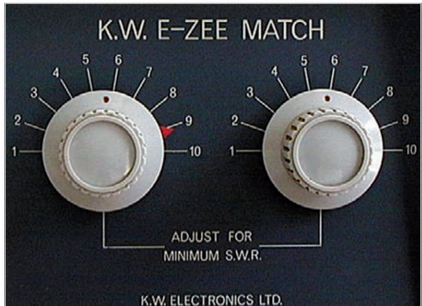
Fig. 3. The KW E-ZEE MATCH can compensate for wide impedance mismatches, but it can be tricky to set up.
